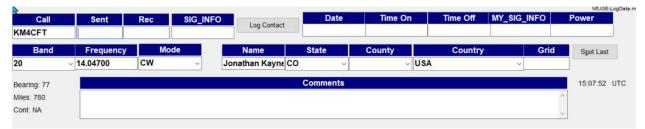
You can also have ACLog interface with your rig to enter the band, frequency and mode as you tune around the bands. The rig interface includes the capability to control the rig using CAT commands. You can setup macros to transmit recorded CW or SSB messages. ACLog, also includes DX spotting from numerous telnet servers. With rig control, you can click on a spot and ACLog will tune your rig and set the correct mode for you to listen in and try to make the contact.
