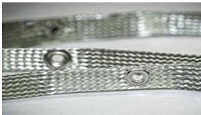
On the manufacturer's website they stated that the purpose for the strap was that it allows for easy attachment of the truck bed to the frame to provide a better "ground plane". That information has been in the back of my mind since I first purchased the ATAS 120. It got tossed aside when the ATAS 120 appeared to work very well with a Breedlove mount. What I didn't realize was that the bed probably lost all grounding over time.
