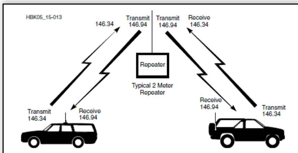
Here is an overall view of a typical 2 meter repeater in operation. The frequencies shown are correct for the Lufkin 94 repeater, but the idea applies to all repeaters.
