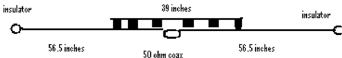
The antenna is fed in the center of the 6 meter element. Cut the 6 meter element at its center and attach an SO-239 with the center conductor connected to one side of the 6 meter wire and the ground connection to the other side. Since this is a balanced antenna with an unbalanced feed line (52 ohm coax) we need to prevent radiation from
