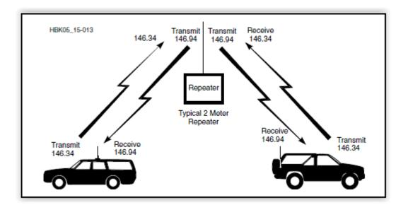
Here is an overall view of a typical 2 meter repeater in operation. The frequencies shown are correct for the Lufkin 94 repeater, but the idea applies to all repeaters.
